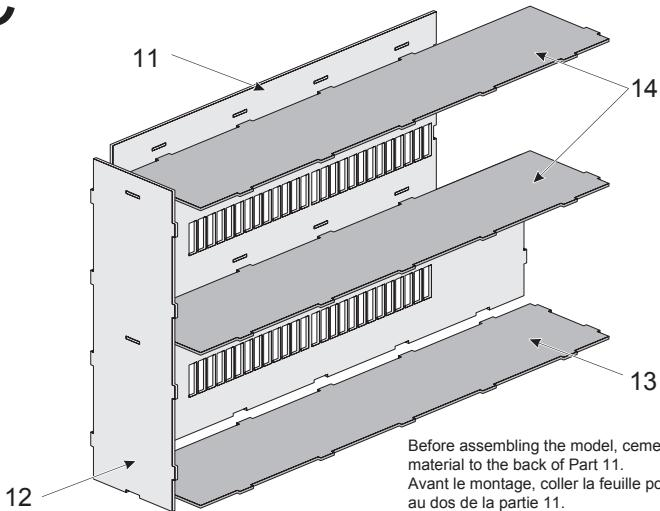
Before assembling the model, cement the window material to the back of Part 11.
