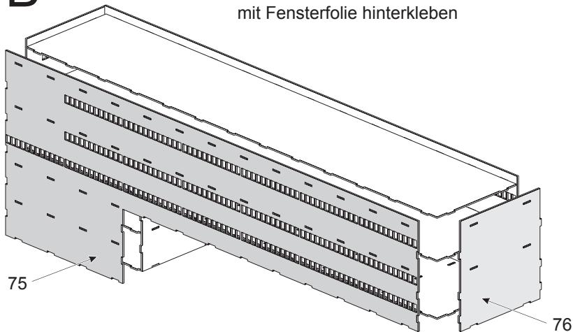
Before assembling the model, cement the window material to the back of Part 75.
