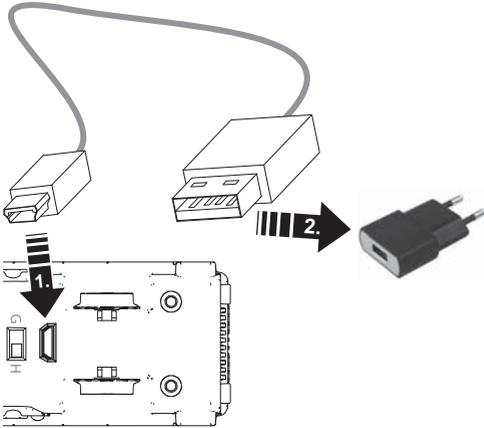
The charging time with the cable included with the train is approximately 3 hours. The train is recharged when the red light in the train goes out.
