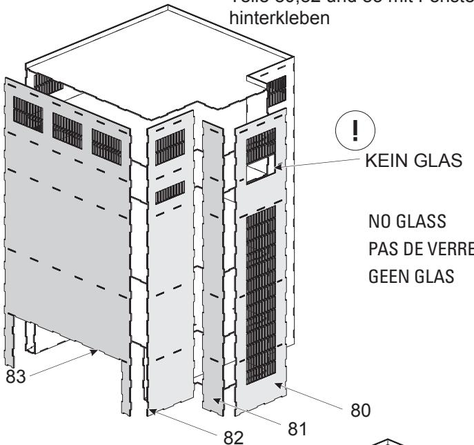
Before assembling the model, cement the window material to the back of Parts 80, 82 and 83.
