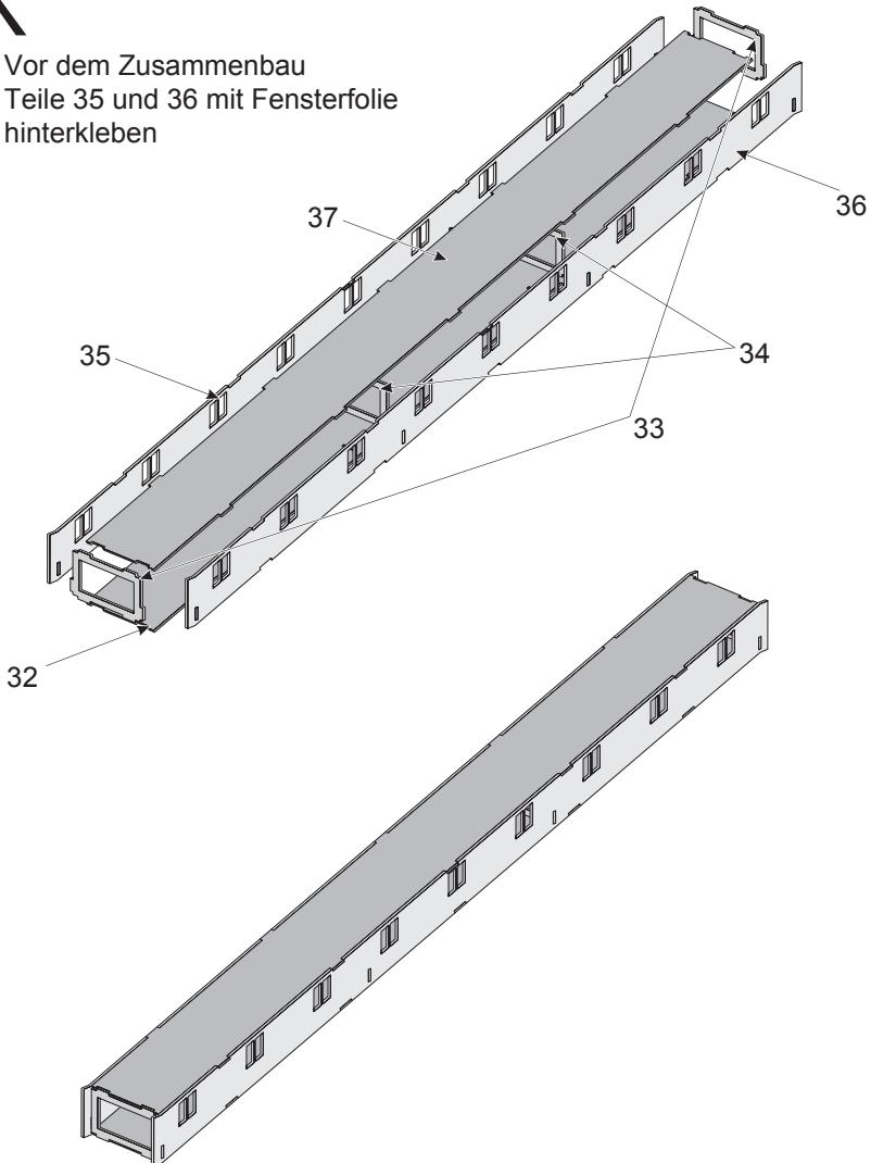
Before assembling the model, cement the window material to the back of Parts 35 and 36.
