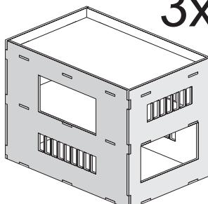
Before assembling the model, cement the window material to the back of Parts 1, 2 and 4.
